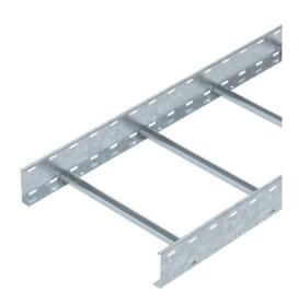
Cable ladder with 110 mm side height with welded C30 profile rungs which are open in an upwards direction. Rolled side rail for reinforcement and as edge protection. Fastening to the bracket takes place using clamps, type LKS 40. The slot dimension of the frame is 16.5 mm and the appropriate U clamp clip is type 2056
