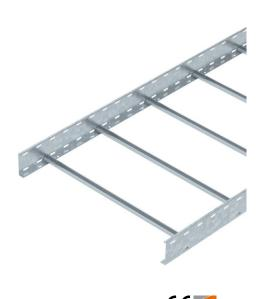
Cable ladder with 110 mm side height with welded C30 profile rungs which are open in an upwards direction. Rolled side rail for reinforcement and as edge protection. Fastening to the bracket takes place using clamps, type LKS 40. The slot dimension of the frame is 16.5 mm and the appropriate U clamp clip is type 2056.
