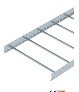
Cable ladder with 110 mm side height with welded C30 profile rungs which are open in an upwards direction. Rolled side rail for reinforcement and as edge protection. Fastening to the bracket takes place using clamps, type LKS 40. The slot dimension of the frame is 16.5 mm and the appropriate U clamp clip is type 2056.
