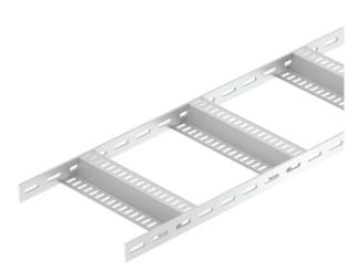
Shipbuilding cable ladder with perforated side rail of side height 40 mm with wel-ded, perforated Z rungs. The shipbuilding cable ladder, including fittings, is also available in stainless steel
