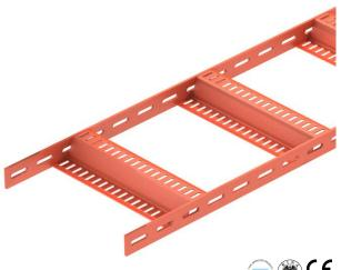
Shipbuilding cable ladder with perforated side rail of side height 40 mm with welded, perforated Z rungs. Load tested according to IEC in conjunction with connector, type SLV. Welding primer type SIGMA-WELD 199, also available in white.
