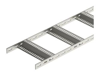
Shipbuilding cable ladder with perforated side rail of side height 40 mm with welded, perforated Z rungs. Load tested according to IEC in conjunction with connector, type SLV.
