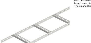
Shipbuilding cable ladder with perforated side rail of side height 25 mm with welded, perforated trapezoidal rungs which open in a downwards direction. Load tested according to IEC in conjunction with connector, type SLV. The shipbuilding cable ladder is also available in unpainted steel on request.
