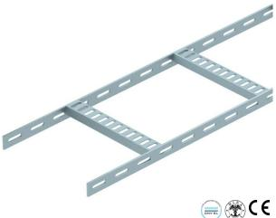
Shipbuilding cable ladder with perforated side rail of side height 25 mm with welded, perforated trapezoidal rungs which open in a downwards direction. Load tested according to IEC in conjunction with connector, type SLV.
