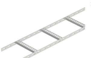
Shipbuilding cable ladder with perforated side rail of side height 25 mm with wel-ded, perforated trapezoidal rungs which open in a downwards direction. Load tested according to IEC in conjunction with connector, type SLV. The shipbuilding cable ladder is also available in unpainted steel on request.
