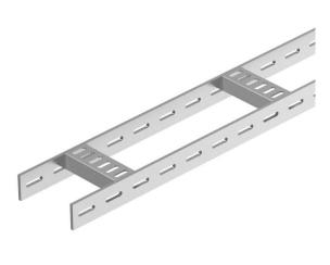
Shipbuilding cable ladder with perforated side rail of side height 40 mm with welded, perforated trapezoidal rungs which open in a downwards direction. Load tested according to IEC in conjunction with connector, type SLV.
