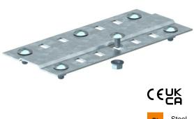
Wide joint plate for use in all cable trays and wide span cable trays. Including appropriate fastening material. For function maintenance at a width of 100 mm, the quantity of supplied M6 truss-head bolts should be increased to four, whilst for widths 200 and 300 mm, it should be increased to six.
