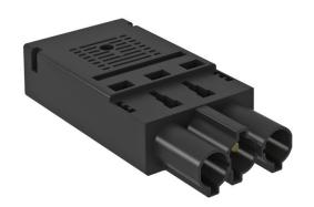
Connector part, 3-pin, type GST18i with spring power connection for rigid cables of 1.5–2.5 mm², single-wire and ultrasonically welded, fine wire cables 1.5 mm² with end sleeves, unmounted with strain relief, can be terminated in situ, 250 V, 16 A.
