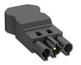
Connector part, 3-pin, type GST18i with screw connection for cables of 1.5–4.0  $\rm mm^2$  and cable diameters between 10.5–14.5 mm (H05VV, NYM), unmounted with strain relief, terminable in situ, 250 V, 16 A.
