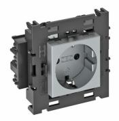
Protective contact socket with connection to side, Single 0°, with increased touch protection, with screwless terminals, 2-pin, 16 A, 250 V~, with connection terminals to IEC 60884-1, suitable for the installation in Rapid 80 device installation trunking system.
