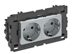
Protective contact socket with connection to side, double 0°, with increased touch protection, with screwless terminals, 2-pin, 16 A, 250 V $\sim$ , with connection terminals to IEC 60884-1, suitable for the installation in Rapid 80 device installation trunking systems.
