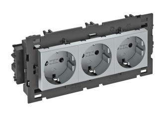
Protective contact socket with connection to side, triple  $0^{\circ}$ , with increased touch protection, with screwless terminals, 2-pin, 16 A, 250 V~, with connection terminals to IEC 60884-1, suitable for the installation in Rapid 80 device installation trunking systems.
