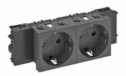
Protective contact socket with connection to side, Double 0°, with increased touch protection, with screwless terminals, 2-pin, 16 A, 250 V $\sim$ , with connection terminals to IEC 60884-1, suitable for the installation in Rapid 45 device installation trunking systems.
