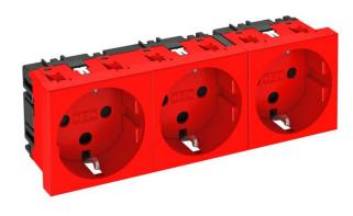
Protective contact socket, triple  $0^\circ$ , encoded version, with increased touch protection, with screwless terminals, 2-pin, 16 A, 250 V~, with connection terminals according to IEC 60884-1.
