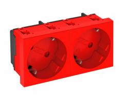
Protective contact socket, double 33°, with increased touch protection, with screwless terminals, 2-pin, 16 A, 250 V $\sim$ , with connection terminals to IEC 60884-1.
