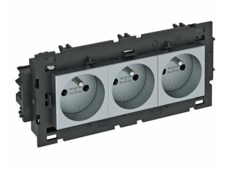
Earthing pin socket with connection to side, Triple  $0^{\circ}$ , with increased touch protection, with screwless terminals, 2-pin, 16 A, 250 V~, with connection terminals to IEC 60884-1, suitable for the installation in Rapid 80 device installation trunking systems.
