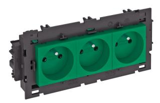
Earthing pin socket with connection to side, Triple  $0^{\circ}$ , with increased touch protection, with screwless terminals, 2-pin, 16 A, 250 V $^{\sim}$ , with connection terminals to IEC 60884-1, suitable for the installation in Rapid 80 device installation trunking systems.
