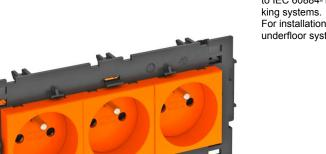
Earthing pin socket with connection to side, Triple 0°, with increased touch protection, with screwless terminals, 2-pin, 16 A, 250 V~, with connection terminals to IEC 60884-1, suitable for the installation in Rapid 80 device installation trunking systems.
