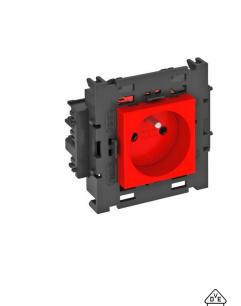
Earthing pin socket with connection to side, Single 0°, with increased touch protection, with screwless terminals, 2-pin, 16 A, 250 V~, with connection terminals to IEC 60884-1, suitable for the installation in Rapid 80 device installation trunking systems.
