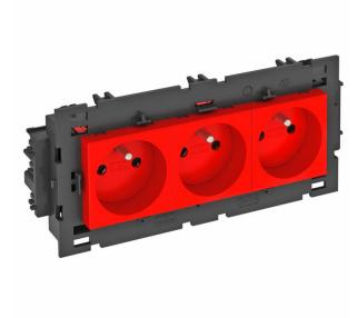
Earthing pin socket with connection to side, Triple  $0^{\circ}$ , with increased touch protection, with screwless terminals, 2-pin, 16 A, 250 V $^{\sim}$ , with connection terminals to IEC 60884-1, suitable for the installation in Rapid 80 device installation trunking systems.
