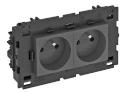
Socket with earthing pin with side connection Double 0°, with increased touch protection with screwless terminals, 2-pin, 16 A, 250 V~, with connection terminals to IEC 60884-1, suitable for installation in Rapid 80 device installation trunking systems.
