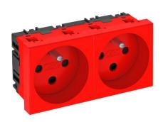
Socket with earthing pin, double  $0^\circ$ , encoded version, with increased touch protection, with screwless terminals, 2-pin, 16 A, 250 V $\sim$ , with connection terminals according to IEC 60884-1.
