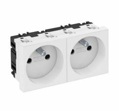
Socket with earthing pin, double  $0^\circ,$  with increased touch protection, with screwless terminals, 2-pin, 16 A, 250 V~, with connection terminals to IEC 60884-1.
