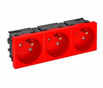
Socket with earthing pin and side connection, Triple 33°, with increased touch protection, with screwless terminals, 2-pin, 16 A, 250 V $\sim$ , with connection terminals to IEC 60884-1.
