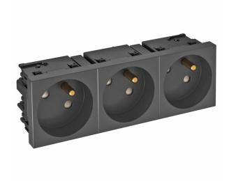
Socket with earthing pin and side connection, Triple 33°, with increased touch protection, with screwless terminals, 2-pin, 16 A, 250 V $\sim$ , with connection terminals to IEC 60884-1.
