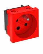
Socket with earthing pin Single 33°, encoded version, with increased touch protection, with screwless terminals, 2-pin, 16 A, 250 V $\sim$ , with connection terminals to IEC 60884-1. The socket can only be used in conjunction with an encoding pin, type CST-STD.
