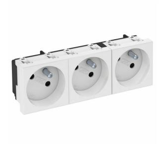
Socket with earthing pin Triple 33°, with increased touch protection, with screwless terminals, 2-pin, 16 A, 250V  $\sim$ , with connection terminals to IEC 60884-1.
