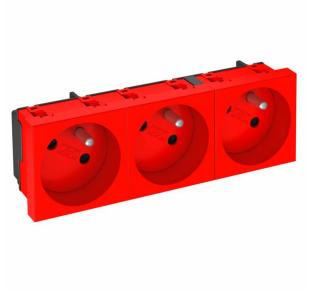
Socket with earthing pin Triple 33°, with increased touch protection, with screwless terminals, 2-pin, 16 A, 250V ~, with connection terminals to IEC 60884-1.
