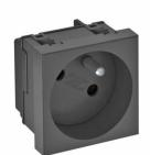
Socket with earthing pin Single 33°, with increased touch protection, with screwless terminals, 2-pin, 16 A, 250V  $\sim$ , with connection terminals to IEC 60884-1.
