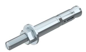
The high-load anchor SZ is a heavy-duty push-through anchor system with a threefold expanding special sleeve which facilitates very high approved loads with small axial spacings and edge distances. The plastic press ring secures the permanent tightening of the fastening piece against the ground.
