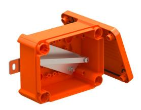
Unequipped, closed connection or junction box for free termination with ceramic terminals and cable glands. Dimension A states the available support rail length for the wiring terminals. Sufficiently large wiring compartment through diagonally arranged support rail. Fastening on easily accessible external flaps made of stainless steel. Approved for cable systems that maintain the electrical function according to DIN 4102 Part 12 with the classes E30, E60 and E90.
