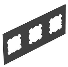
Cover plate with 3 perforations ( $\varnothing$  45 mm) for three accessories with support ring or bracket, suitable for T12L lengthwise side (3/4 cover).
