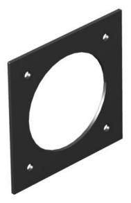
Cover plate with 1 perforation ( $\varnothing$  70 mm) and 60 x 60 mm screw fastening for CEE sockets, suitable for T4L and T8NL narrow side or for T4L and T8NL lengthwise side (1/2 cover).
