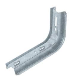
TP bracket with clamping lugs. If the bracket is fastened directly to the wall or the profiles are screwed together, then, for reasons of stability, always use the spacer, type DS 4. Mesh cable trays with a 50 x 100 mm grid width, e.g. type GRL, GR and GRM, can be fastened to the TP bracket without screws.
