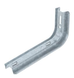
TP bracket with clamping lugs. If the bracket is fastened directly to the wall or the profiles are screwed together, then, for reasons of stability, always use the spacer, type DS 4. Mesh cable trays with a 50 x 100 mm grid width, e.g. type GRL, GR and GRM, can be fastened to the TP bracket without screws.
