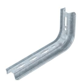
TP support/bracket for fastening to horizontal concrete ceilings and walls. If the profile is fastened directly to the ceiling or the profile is screwed together as head reinforcement, then, for reasons of stability, always use the spacer, type DS
