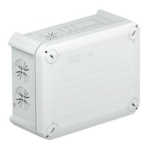
Junction box for 4 Wieland sockets, 3-5-pin, for the connection of cables indoors and in protected outdoor areas. Rectangular design with knock-out entries to the sides and knock-out entries in the bottom. Suitable for wall and ceiling mounting and on mounting panels. With the option of fastening inside and to mount via the corner domes. Cover with quick lock, sealable. Made from halogen-free and UVresistant materials.
