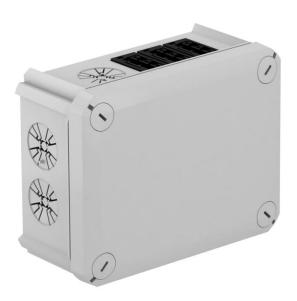
Junction box with WAGO sockets, 3-pin. 6x black for the connection of cables indoors and in protected outdoor areas. Rectangular design with knock-out entries to the sides and knock-out entries in the bottom. Suitable for wall and ceiling mounting and on mounting panels. With the option of fastening inside and to mount via the corner domes. Cover with quick lock, sealable. Made from halogen-free and UV-resistant materials.
