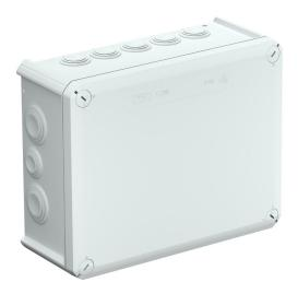
Junction box for the connection of cables and lines indoors and in protected outdoor areas. Rectangular design with plug-in seals to the sides and knock-out entries in the bottom. Suitable for wall and ceiling mounting, on mounting panels and threads in the floor. With the option to fasten inside and to mount via the corner domes. Cover with quick lock, sealable. Made from halogen-free materials. Flame-resistant type made from special polypropylene.
