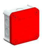
Junction box for the connection of cables and lines indoors and in protected outdoor areas. Square design with knock-out entries to the sides and knock-out entries in the bottom. Suitable for wall and ceiling mounting and on mounting panels. With the option to fasten inside and to mount via the corner domes. With fixed clamping cover. Made from halogen-free and UV-resistant materials.
