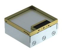
Square installation unit for use in dry-care cavity and screed floors for indoor use. Installation housing with pre-marked insertion openings for pipelines (M25). Cable outlet via brush bar in hinged lid. Cover adjustable to top edge of floor covering using four height adjustment supports. 15 mm floor covering recess in the hinged lid. The minimum installation depth is 95 mm, the height adjustment range + 30 mm.
