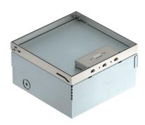
Square floor box for four installation devices of Italian design, for use in dry-care cavity and screed floors for indoor use. Installation housing with pre-marked insertion openings for pipelines (M25). Cover adjustable to top edge of floor covering using four height-adjustment supports. 15 mm floor covering recess in the hinged cover. The minimum installation depth is 110 mm, the height-adjustment range + 30 mm.
