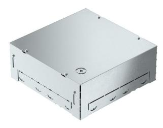
Square installation housing for one GES9-2 service outlet for the use in screed floors for indoor use. With pre-marked insertion openings for pipelines (M25) on all four sides
