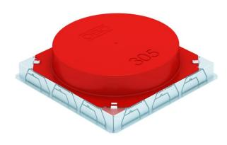
Underfloor outlet box with fixed, unchangeable installation opening of  $\varnothing$  305 mm for an installation unit of nominal size R9. The mounting opening is created using the screed protection cover contained in the scope of supply. The underfloor box possesses installation openings for three single-compartment PVC ducts of nominal size 60 x 25 and 90 x 35 on all four sides. The box is principally suited for use in floor structures in cement screed with a structure height of up to 95 mm.
