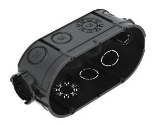
Double flush-mounted device box, for use in masonry with an installation depth of at least 46 mm.
