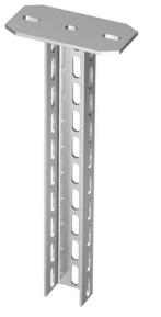
Suspended support (U profile) with welded head plate. For fastening to horizontal concrete ceilings and steel girders. For bracket widths of 400 mm or more, or if the bracket is mounted at the end of a suspended support, we recommend the use of the spacer, type DSK 61.
